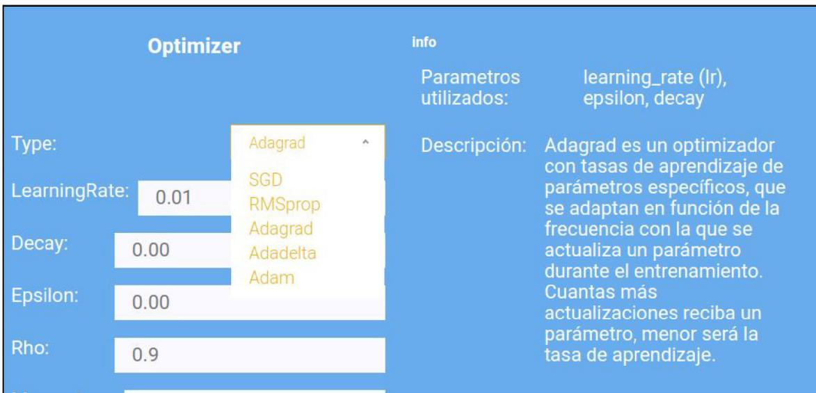
The screenshot shows the 'Optimizer' section of the configuration interface. The 'Type' dropdown menu is open, showing a list of optimizers: Adagrad (selected), SGD, RMSprop, Adagrad, Adadelta, and Adam. The other parameters (LearningRate: 0.01, Decay: 0.00, Epsilon: 0.00, Rho: 0.9) are visible below the dropdown. The 'Info' section on the right provides the same description as in Figure 29.
